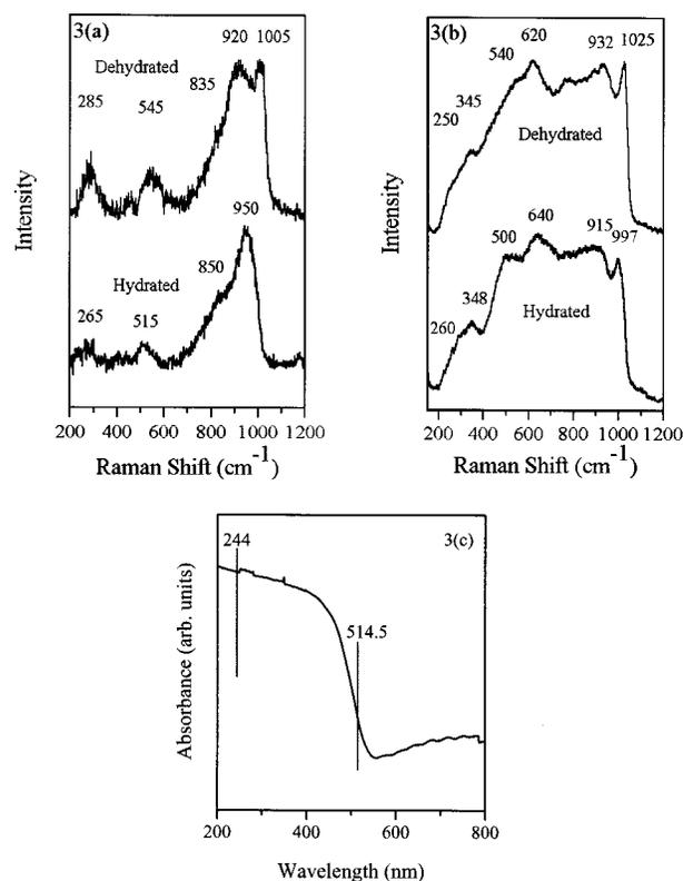
**Figure 3.** (a) UV Raman spectra of hydrated and dehydrated 20%  $\text{V}_2\text{O}_5/\text{Al}_2\text{O}_3$  (monolayer). (b) Visible Raman spectra of hydrated and dehydrated 20%  $\text{V}_2\text{O}_5/\text{Al}_2\text{O}_3$  (monolayer). (c) UV-visible diffuse reflectance spectra of hydrated 20%  $\text{V}_2\text{O}_5/\text{Al}_2\text{O}_3$  (monolayer).
