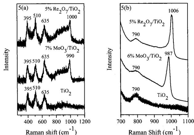
**Figure 5.** (a) UV Raman spectra of TiO<sub>2</sub> (anatase), dehydrated 7% MoO<sub>3</sub>/TiO<sub>2</sub> (monolayer), dehydrated 5% Re<sub>2</sub>O<sub>7</sub>/TiO<sub>2</sub>. (b) Visible Raman spectra of TiO<sub>2</sub> (anatase), dehydrated 6% MoO<sub>3</sub>/TiO<sub>2</sub> (monolayer), dehydrated 5% Re<sub>2</sub>O<sub>7</sub>/TiO<sub>2</sub>.
