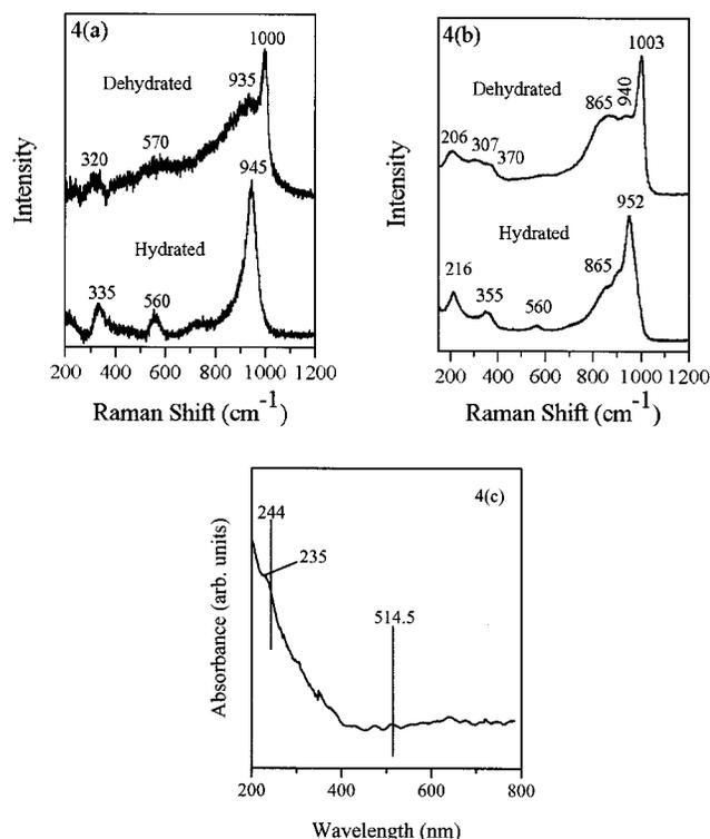
**Figure 4.** (a) UV Raman spectra of hydrated and dehydrated 18% MoO<sub>3</sub>/Al<sub>2</sub>O<sub>3</sub> (monolayer). (b) Visible Raman spectra of hydrated and dehydrated 18% MoO<sub>3</sub>/Al<sub>2</sub>O<sub>3</sub> (monolayer).
