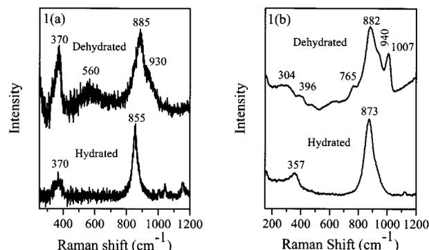
**Figure 1.** (a) UV Raman spectra of hydrated and dehydrated 0.5% CrO<sub>3</sub>/Al<sub>2</sub>O<sub>3</sub>. (b) Visible Raman spectra of hydrated and dehydrated 0.5% CrO<sub>3</sub>/Al<sub>2</sub>O<sub>3</sub>.
