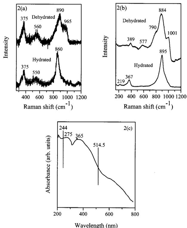
**Figure 2.** (a) UV Raman spectra of hydrated and dehydrated 5%  $\text{CrO}_3/\text{Al}_2\text{O}_3$ . (b) Visible Raman spectra of hydrated and dehydrated 5%  $\text{CrO}_3/\text{Al}_2\text{O}_3$ . (c) UV–visible diffuse reflectance spectra of hydrated 5%  $\text{CrO}_3/\text{Al}_2\text{O}_3$ .
